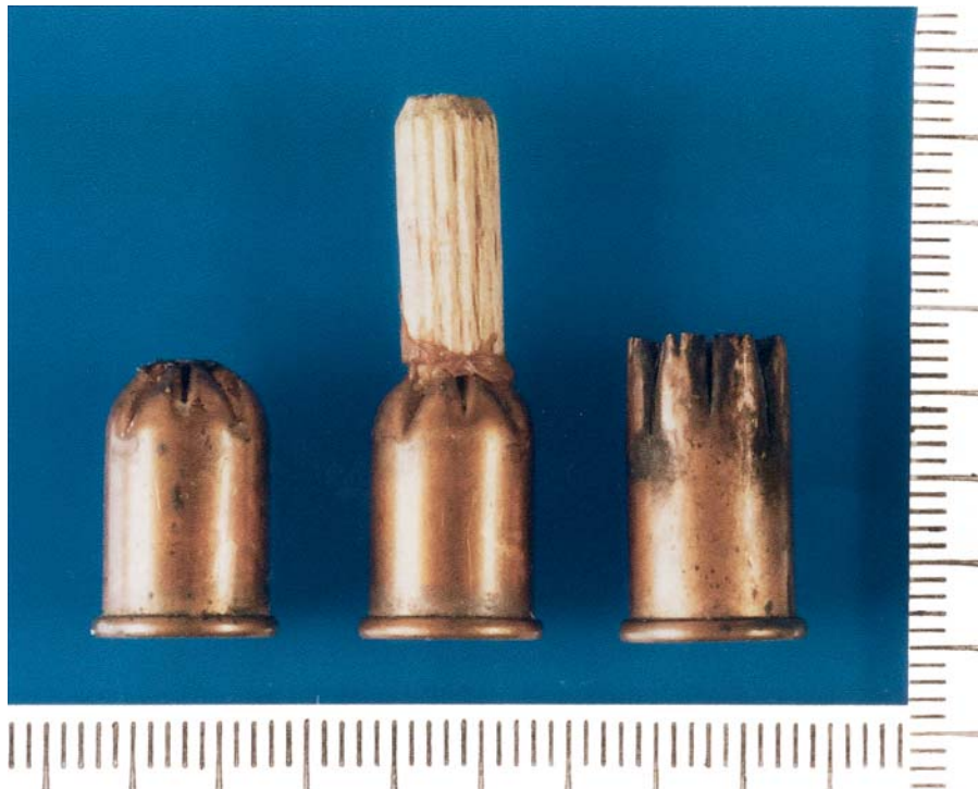
FIG. 2—Ammunition used in the presented case. Blank cartridges 17 mm × 9, cal. .380. Left: blank cartridge, middle: a wooden dowel had been glued on top the otherwise nonmanipulated cartridge, right: expended manipulated cartridge found in the cylinder. Self-constructed ammunition: wooden dowel glued on top a conventional cal. .380 blank cartridge. Note traces of adhesive substance, most probably a synthetic resin compound on the dowel.
