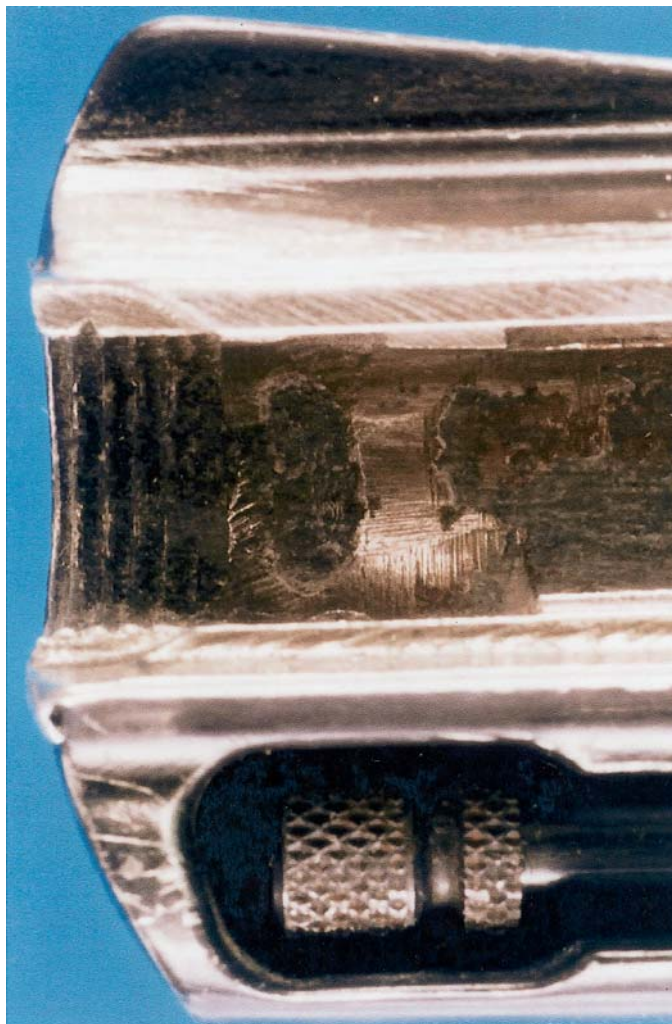
FIG. 5—Manipulated barrel showing fine longitudinal traces of mill cutting in proximity to the muzzle (detailed view). Note thread for insertion of adapter devices for the use of signal ammunition.
